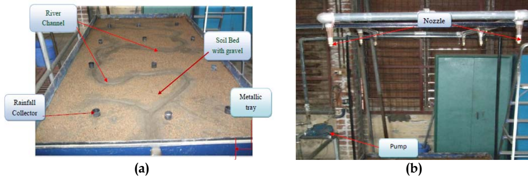
Fig. 1. Components of the hydrology bench: (a) soil filled metallic tray and (b) rainfall simulator
