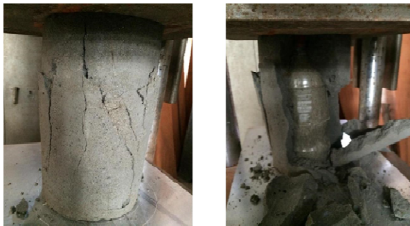
Figure 4. Plastic bottle filled cylinder during compressive strength test and after complete failure.
