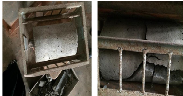
Figure 5. The plastic bottle brick filled cylinder assembled for split tensile strength test and the cylinder after failure.
