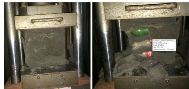
Figure 6. Plastic bottle filled cubes during compressive strength test and after complete failure.
