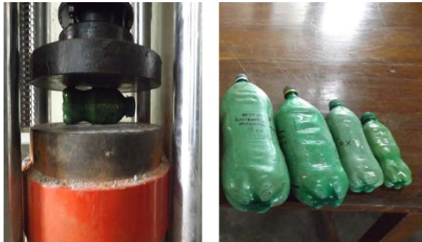
Figure 3. Compression test for plastic bottle bricks and deformed bricks after the test.
