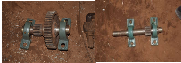
Figure 8. Idle shaft and line shaft.
