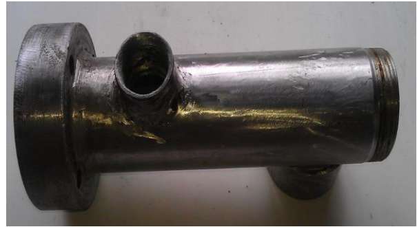
Figure 4. Photographic view of pressure case cylinder.
