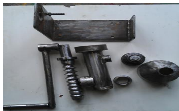
Figure 14. Different parts of manually operated oil palm crusher (all dimensions are in cm).
