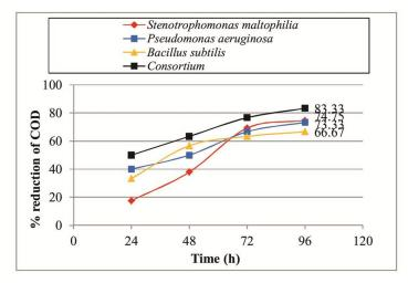
Fig. 5. Wastewater treatment using monoculture and consortium.
