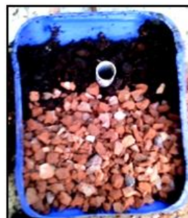
Figure 8. Mixture of Brick lets and used tea leaves media
