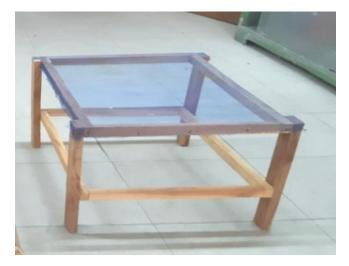
Figure 2. Open sun rack dryer
