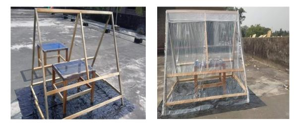
Figure 1. Solar tent dryer without polythene sheet and with polythene sheet
