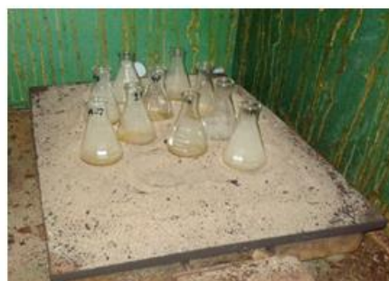
Figure 4. White fume evolves after completion of digestion on sand bath
