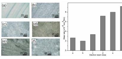
Fig. 2. Optical microscopic images of the worn surfaces at sliding tracks on POM-C surfaces with x20 resolution: (a) unirradiated POM-C; (b) 100 kGy; (c) 200 kGy; (d) 300 kGy; (e) 500 kGy and (f) 700 kGy electron beam dose irradiated surfaces. Scale bar 25  $\mu$ m in each case.
