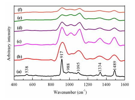
Fig. 7. Raman spectra demonstrating the chemical structural modification due to electron beam dose irradiation on POM-C surfaces: (a) unirradiated; (b) 100 kGy; (c) 200 kGy; (d) 300 kGy; (e) 500 kGy and (f) 700 kGy.
