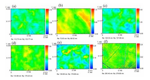
Fig. 8. 2D surface profile images on POM-C samples at 20x objective: (a) unirradiated; (b) 100 kGy; (c) 200 kGy; (d) 300 kGy; (e) 500 kGy and (f) 700 kGy.
