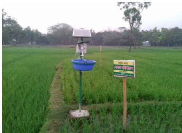
Figure 2. Experimental setup of solar light trap at T-Aman rice field in Barhatta Upazila of Netrokona district
