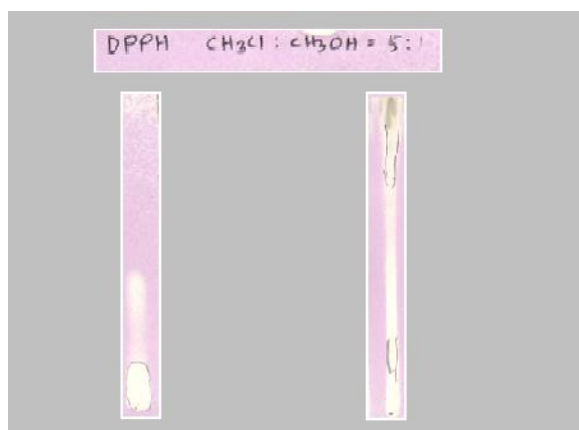
Figure 1. Medium polar solvent applied and DPPH treated Ascorbic Acid and Vallaris solanacea (Roth) Kuntze.
